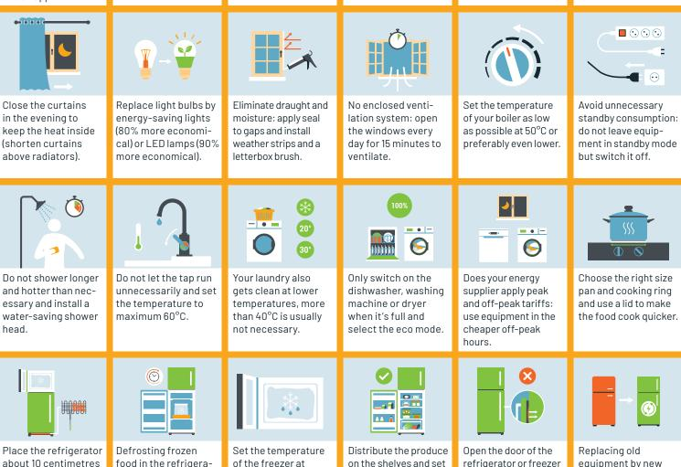
Place the refrigerator about 10 centimetres off the wall and keep the condensation arid dust-free.
